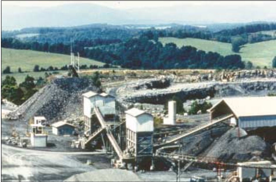
Figure 10. Engineering techniques, such as enclosing equipment and removing dust using vacuums, can mitigate impacts of noise and dust. (Photograph courtesy of Luck Stone.)
