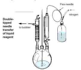
Most researchers only need to use small quantities, so the syringe method works best. Be cautious with the use of the plastic syringe as the rubber gasket may swell up leaving you with a syringe of pyrophoric liquid. Start with small quantities, until you are proficient with the method.
